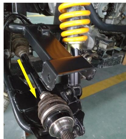
3. Inspect the shaft splines and cv boots for any damage.
