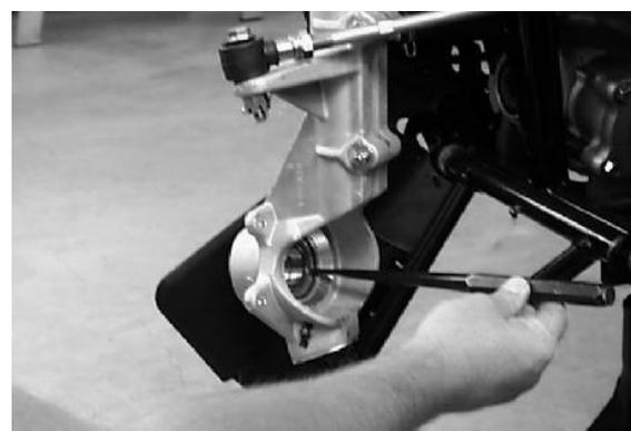
5. Inspect bearing housing for scratches, wear or damage. Replace housing if damaged.
