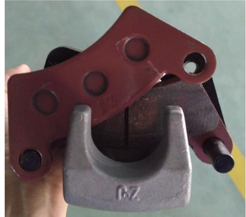
3. Lubricate mounting bracket pins with a light film of All Season Grease, and install rubber dust boots.
