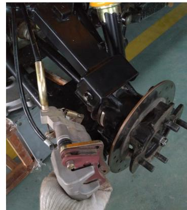
5. Loosen two bolts that secure the rear knuckle to the A-arm. Remove the rear knuckle assembly by sliding it off of the axle.
