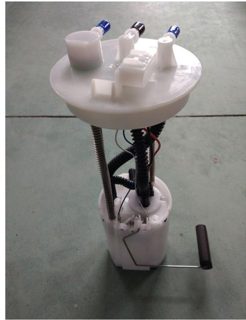
**Fuel Gauge / Fuel level Sensor Inspection**
